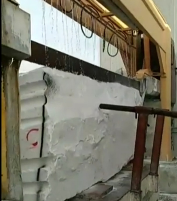
Initial cutting of the Carrara block Pietrasanta, Italy
